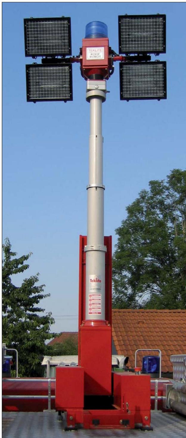
Model RRTM1 with 4 x 1000 Watt Halogen lamps
