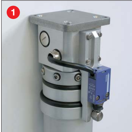
1 Mast top assembly with 1 x PG9, 1 x PG11, 1 x PG13,5 cable gland and 8 mm top flange fitted to keyed mast sections
