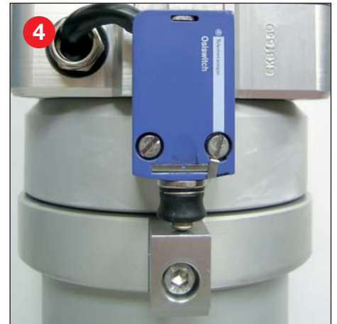
4 Standard pre-mounted and connected warning switch
